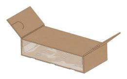
Fold the flaps of the Lid Box onto the Lid Plate.
